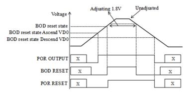
Fig. 4. Relations between power-on reset and brown-out detection
