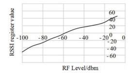
Fig. 2. Relation between RSSI value and input power
